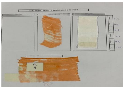
Figure 08: Fastness test result, Silk sample
