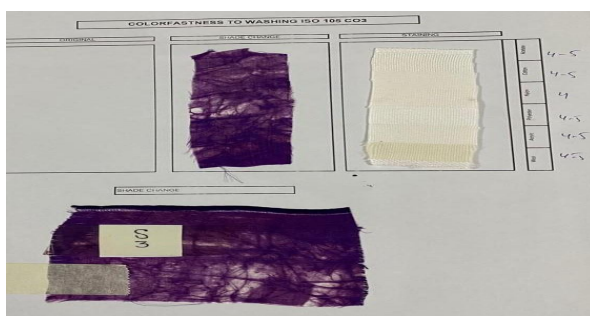
Figure 10: Washing fastness test result, Silk sample
